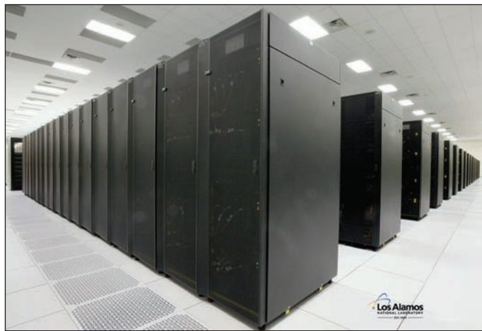
▲ ROADRUNNER. The Roadrunner supercomputer, developed by IBM, operates at speeds exceeding one petaflop, or a thousand trillion calculations per second, roughly equivalent to the combined computing power of 100,000 of the world's fastest laptop computers.
