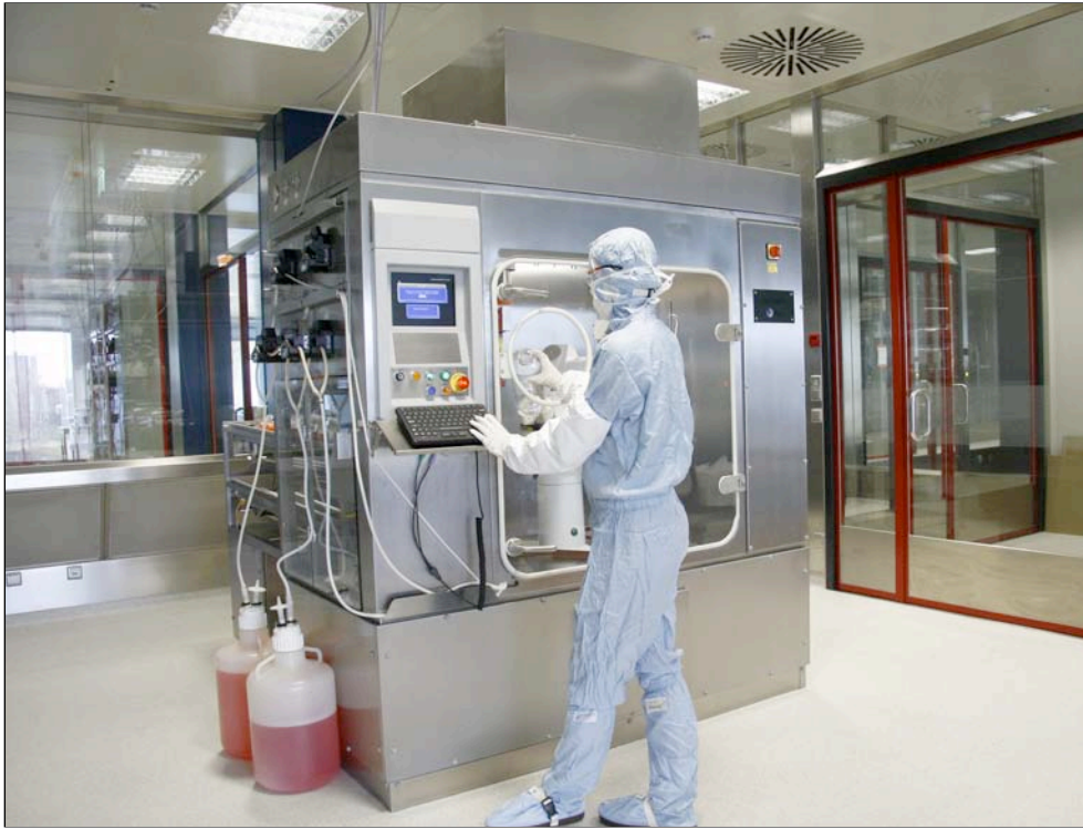
A laboratory worker at the German vaccine manufacturer IDT handles a roller bottle to be filled by a robot with sterile cell cultures containing modified vaccinia Ankara (MVA) vector and growth media.
